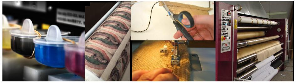
Even though the production technique is relatively simple, It's the chemical process that differentiates sublimation from any other form of textile printing; when sublimation inks are heated over 380 F they turn into gas and form a permanent bond.
